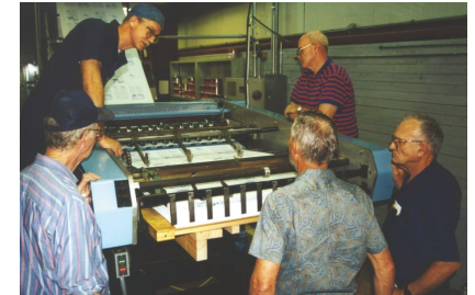
Philip Fraiser and Crew Evaluating Efficiency with a Sheeter Attachment for the Color King Press. — Photo by SLM Archives
